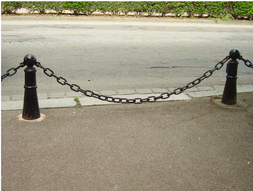
Figure 2.4: The catenary is the shape of a heavy chain suspended at its ends. Image from Wikipedia .
